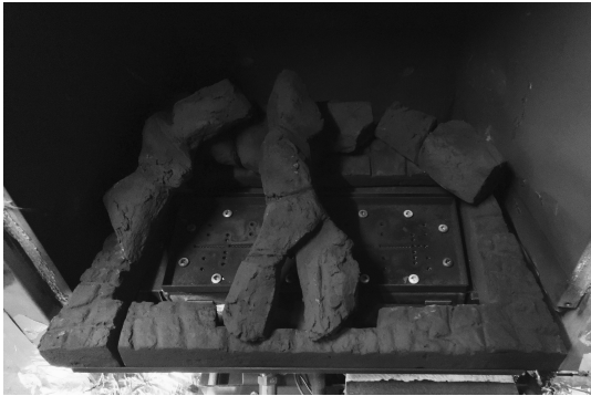
left The centre coal piece has a branch to allow pilot light to be seen position this to allow enough of pilot to be on show
