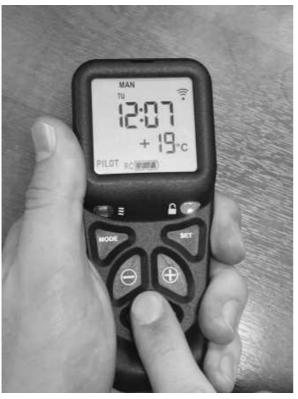
Press and hold in the power symbol button and release immediately when the word pilot comes on to the display at the bottom left as shown (about 1-2 seconds). The stove will light. (NOTE: Releasing too soon or too long after the pilot illumination, results in the fire not lighting, this is for safety reasons).
