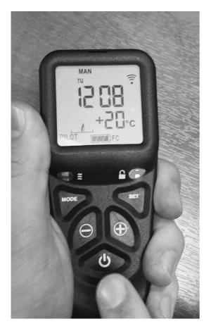
Hold the handset as shown, wrapping your hand around the handset touching both sides. In a second or less the green unlock light will illuminate, allowing the buttons to work when pushed. (NOTE: If the green light is not a constant green or not lit at all the buttons will not be operable).
