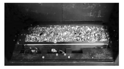
Completely fill the burner with the mica supplied Ensure if any spills into pilot it is removed
