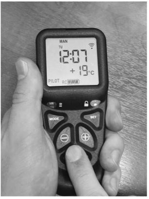
Press and hold in the power symbol button and release immediately when the word pilot comes on to the display at the bottom left as shown (about 1-2 seconds). The stove will light.
