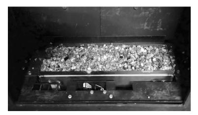
Completely fill the burner with the mica supplied Ensure if any spills into pilot it is removed
