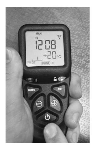
Hold the handset as shown, wrapping your hand around the handset touching both sides. In a second or less the green unlock light will illuminate, allowing the buttons to work when pushed.
