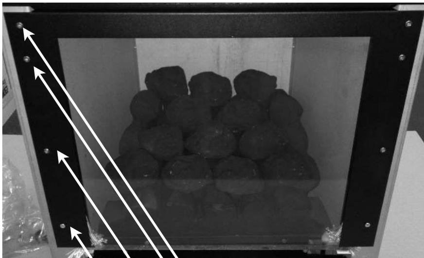
Remove 8 glass cover fixing screws 4 on each side ,left hand side shown above
