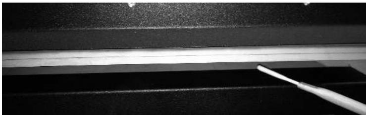
Insert smoke match into Diverter as shown just Above glass cover
