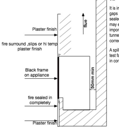
It is important when installing the convector box that all gaps around the inside of the fireplace opening are sealed .the base both sides left and right and the rear may even need pointing in between the brickwork it is important that the flue can only pull through the flue tunnel for the appliance to clear its products and work correctly
