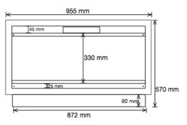
THE CONNELLY CURVE HAS A 25 MM AIR INLET ON THE FRONT OF THE APPLIANCE BENEATH THE GLASS FRAME **UNDER NO CIRCUMSTANCES SHOULD THIS EVER BE BLOCKED OFF OR COVERED**
