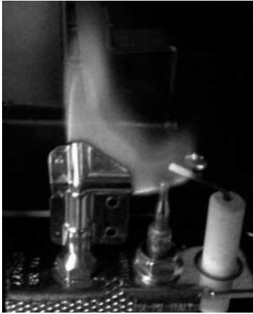
Left strong blue pilot this is correct & safe
