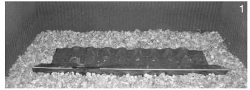
spread the granules around the base WARNING DO NOT BLOCK AIR RELIEF AT FRONT AND BACK OF BURNER
